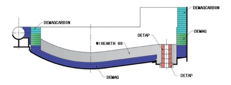
DEMAGCARBON Series - Magnesia carbon brick (any carbon content available upon request)
