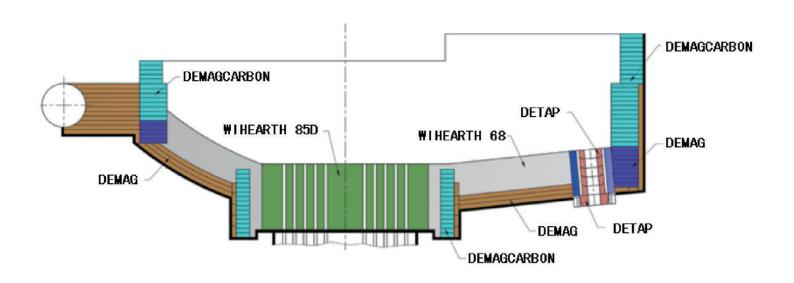
DEMAGCARBON Series – Magnesia carbon brick (any carbon content available upon request)
